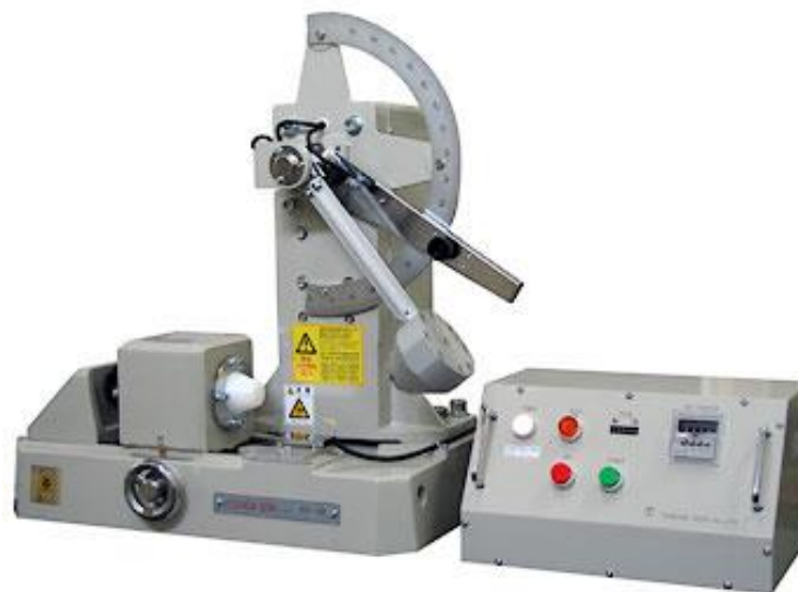
Figure 4 - Pendulum shock testing apparatus [10]
